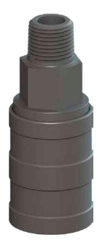
The PVC Quick Disconnect Coupling is available on select retractable and non-retractable quills. It provides a dry-break method of rapidly connecting or disconnecting the chemical feed from the inlet of the quill. This proves to be an invaluable time saver for applications such as sodium hypochlorite where more frequent maintenance cycles might occur.
