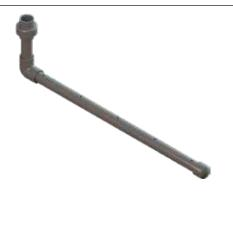
OCDL diffusers allow for two mounting options. Typically, the diffuser would be mounted to a channel wall, parallel to the flow, with the chemical being discharged away from the wall and into the process flow. However with adequate support<sup>4</sup>, the OCDL can also be mounted perpendicular to the flow, spanning the channel, similar to the OCDT. Either configuration can provide a simple, straightforward means of introducing chemical into open channel process flows.
